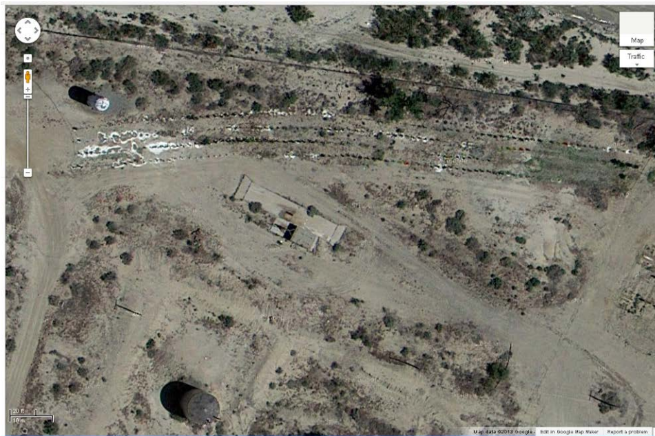
Figure 22. Satellite image of phytoremediation site in Bloomfield, NM showing Phase 1 plantings in four long rows along the north perimeter of the refinery. Note the salt and iron deposits clearly visible in the downstream areas of the dripline on the west side of the site (Google, 2013). Despite the difficult growing environment, poplars have shown adequate growth and health.
